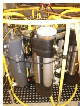
**Figure 18:** CTD with regular free-flow bottles (left) and new AFIS (right). Photo: C. Bannock
