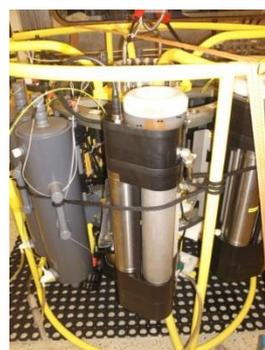
**Figure 18:** CTD with regular free-flow bottles (left) and new AFIS (right). Photo: C. Bannke
