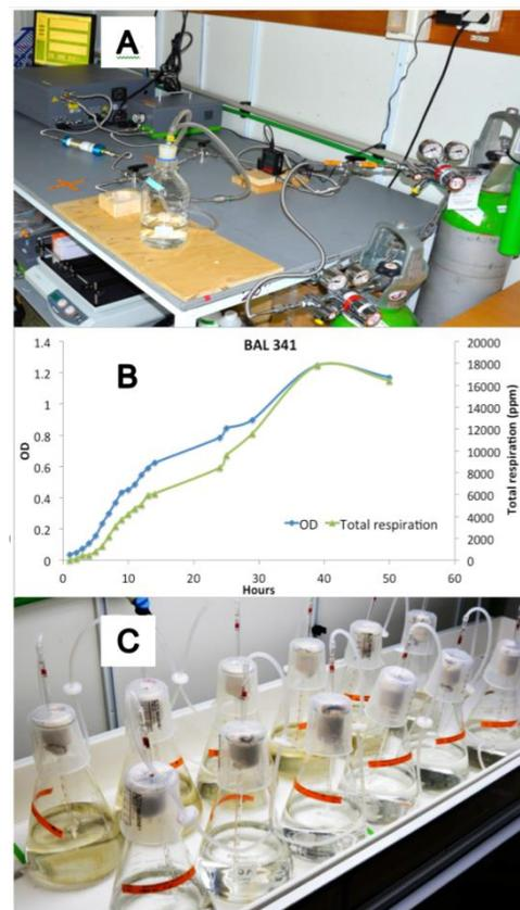
**Figure 8:** Technical setup for the Picarro  $\delta^{13}\text{C}$  carbon dioxide analyzer (A). Growth performance results for heterotrophic Baltic Sea model bacteria using Picarro (B). Model bacteria growing in organic matter from different phytoplankton species (C).
