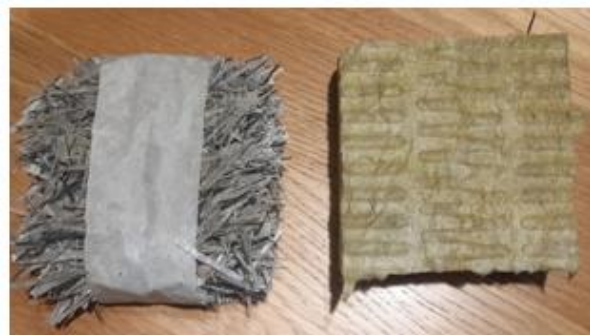
Figure 1. The two materials used in the experiment. Left: the recycled composite material with low density; Right: high density mineral wool
