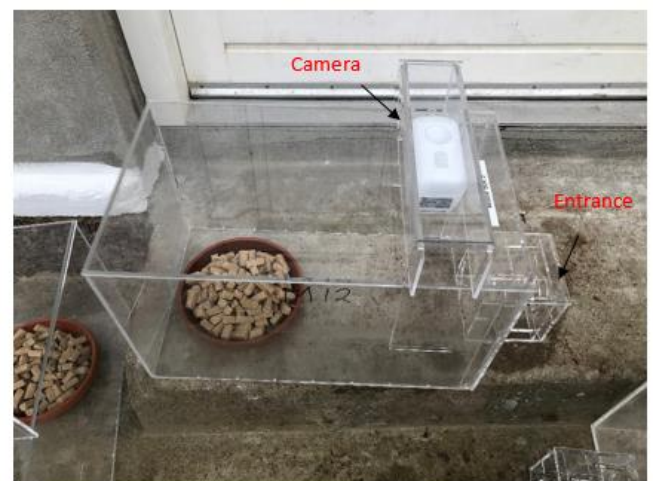
Figure 2: Box out of plexiglass. The camera slot is on top and the entrance on the right. The food (nutrition pallets) is placed in a bowl inside of the box.
